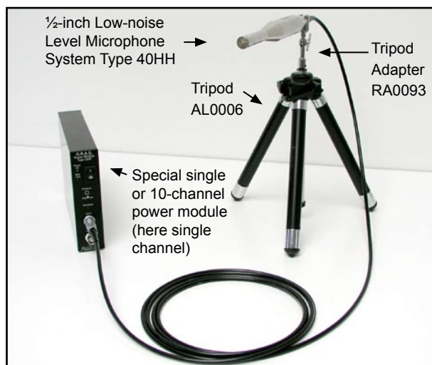
Fig. 2 A complete single-channel low-noise level measuring system
