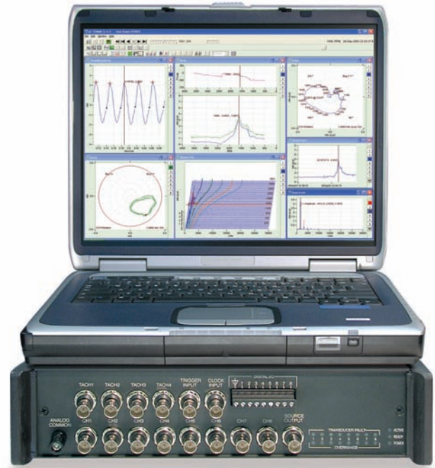
View Time-Domain, Spectrum, Waterfall, and Trend simultaneously on one screen with eZ-TOMAS
